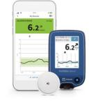
The small, discreet sensor worn on the back of the upper arm continuously measures the glucose concentration in the body's interstitial fluid. It is worn for up to 14 days and is water-resistant so continues to work while you shower, swim or exercise.<sup>4</sup>
